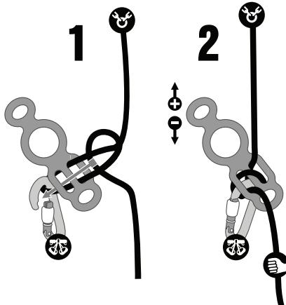
AutoBlock Plaquette mode can be used for ascending or tensioning a rope.
